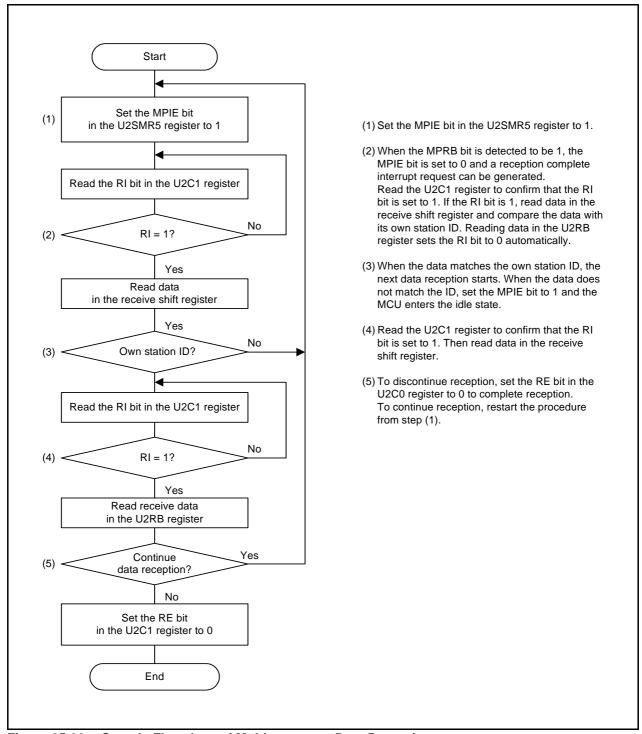
Figure 25.20 Sample Flowchart of Multiprocessor Data Reception
