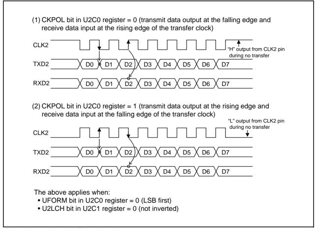
Figure 25.4 Transfer Clock Polarity
