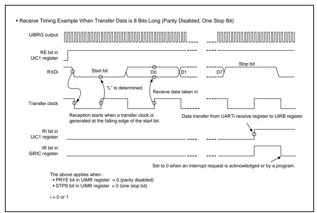
Figure 24.7 Receive Timing in UART Mode
