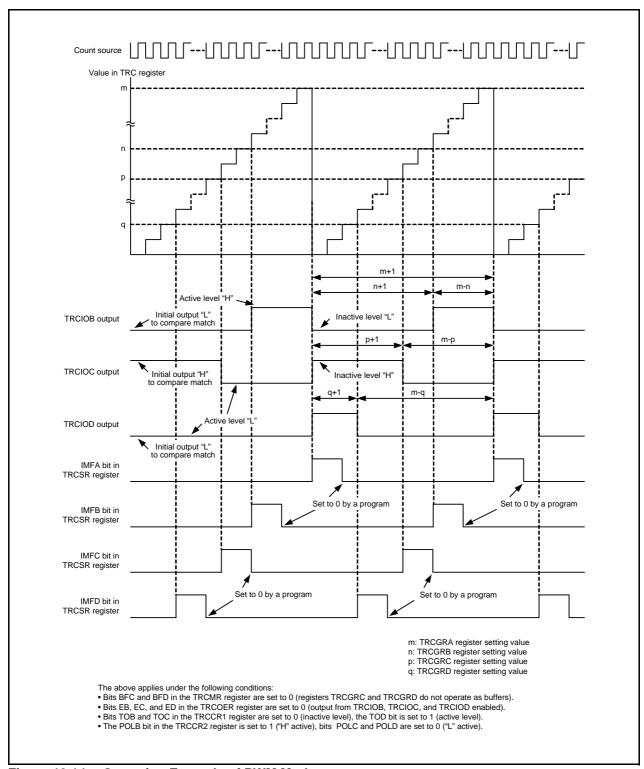
Figure 19.14 Operating Example of PWM Mode
