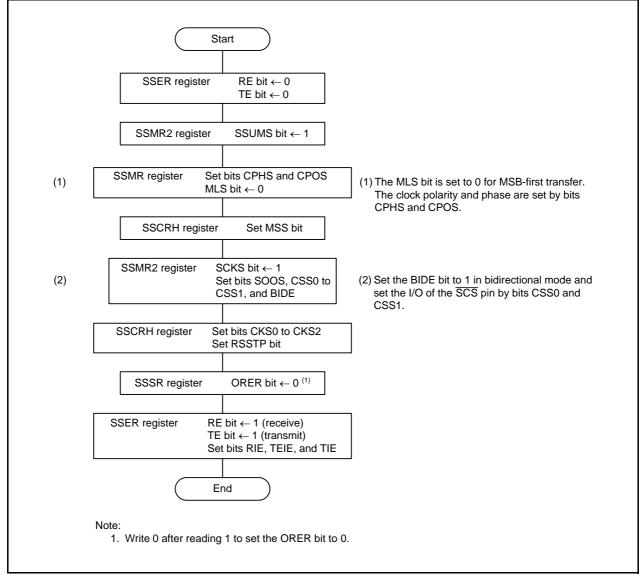
Figure 27.10 Initialization in 4-Wire Bus Communication Mode
