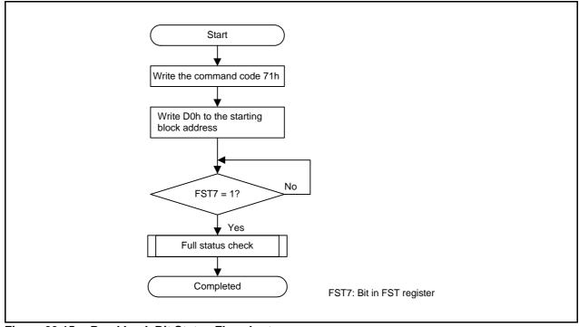
Figure 33.15 Read Lock Bit Status Flowchart
