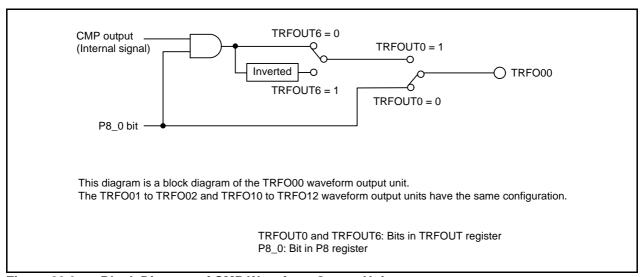
Figure 22.3 Block Diagram of CMP Waveform Output Unit
