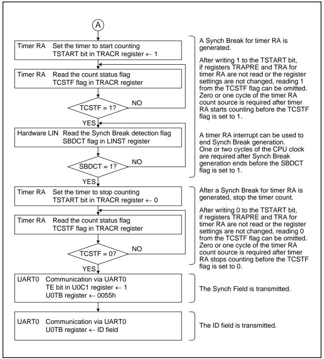
Figure 29.4 Header Field Transmission Flowchart Example (2)
