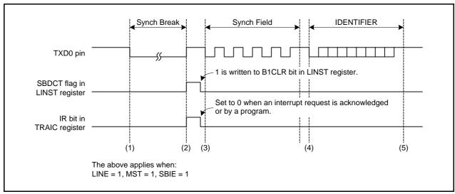
Figure 29.2 Operating Example during Header Field Transmission
