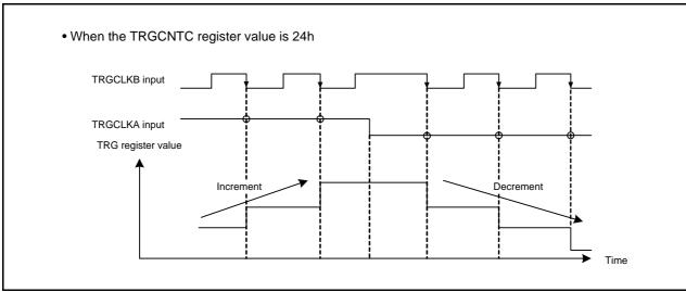
Figure 23.18 Operating Example 2 in Phase Counting Mode
