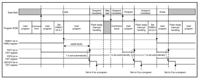
Figure 33.4 Suspend Operation Timing
