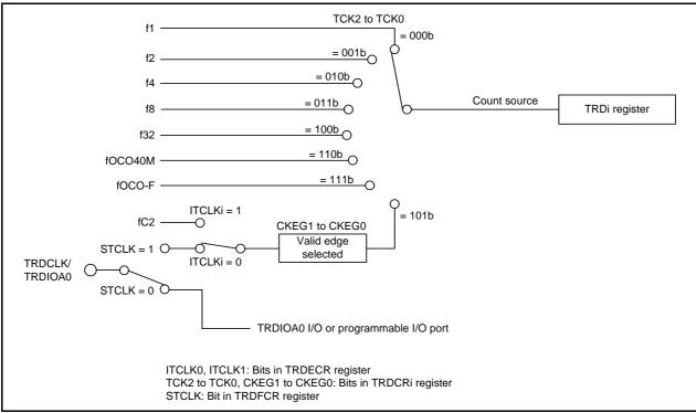
Figure 20.2 Block Diagram of Count Source
