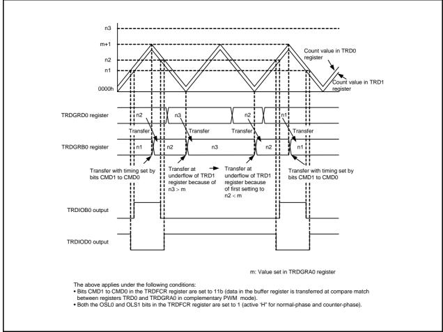
Figure 36.4 Operation when Value in Buffer Register ≥ Value in TRDGRA0 Register in Complementary PWM Mode
