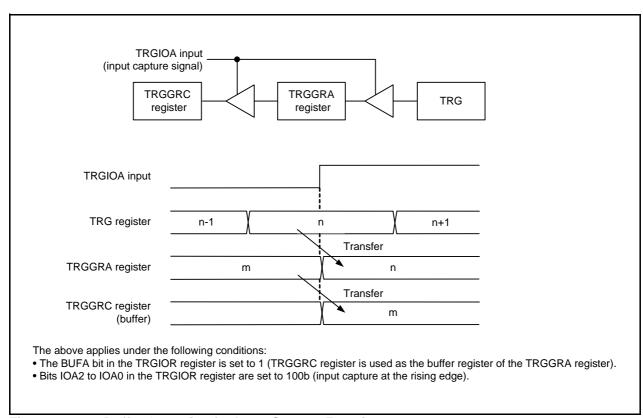
Figure 23.3 Buffer Operation for Input Capture Function
