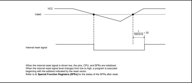
Figure 6.5 Operating Example of Voltage Monitor 0 Reset
