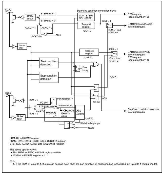
Figure 25.13 I<sup>2</sup>C Mode Block Diagram
