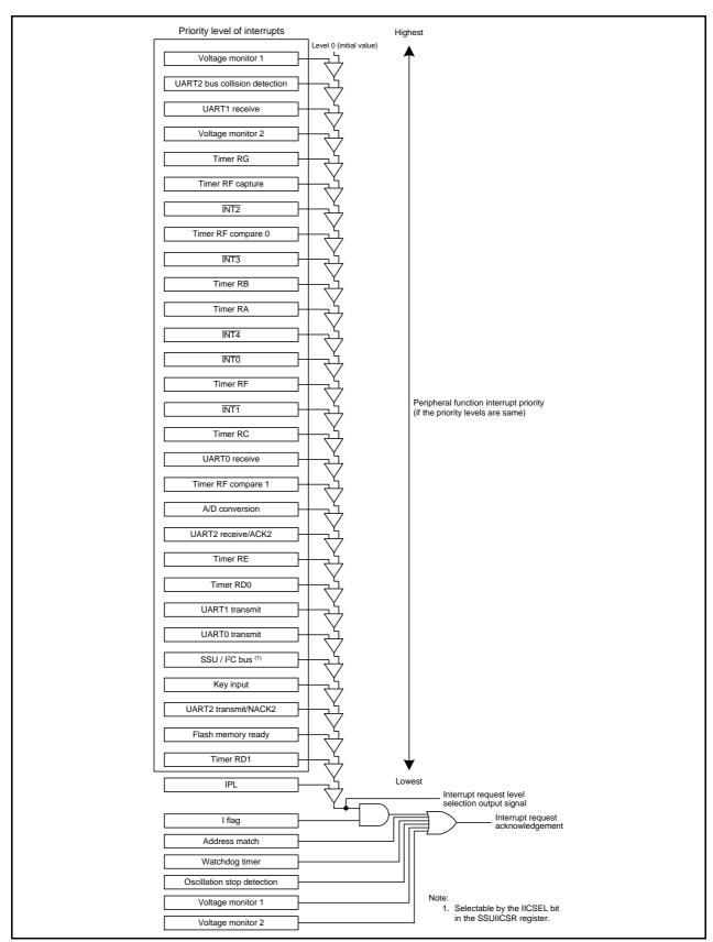
Figure 11.8 Interrupt Priority Level Selection Circuit
