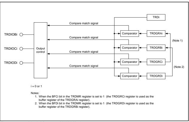
Figure 20.14 Block Diagram of PWM Mode
