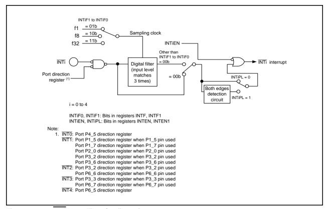
Figure 11.9 INTi Input Filter Configuration
