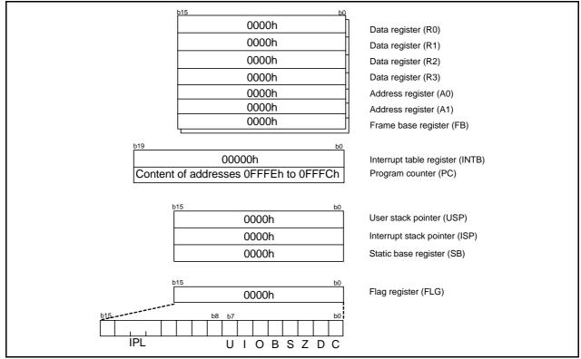
Figure 5.2 CPU Register Status after Reset
