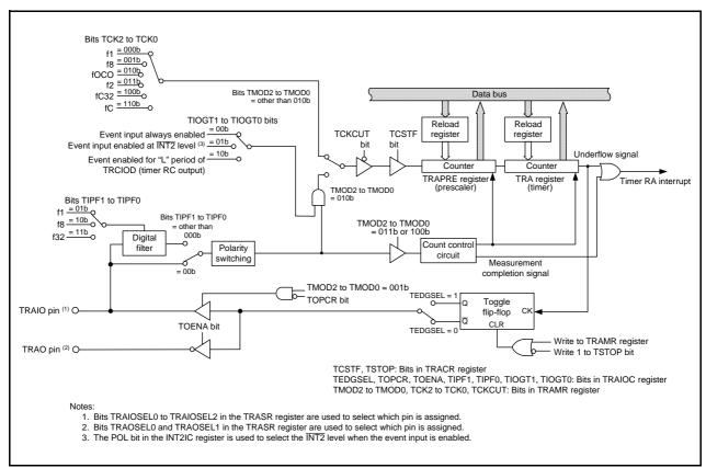
Figure 17.1 Timer RA Block Diagram
