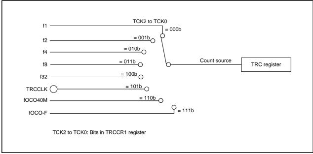
Figure 19.2 Count Source Block Diagram
