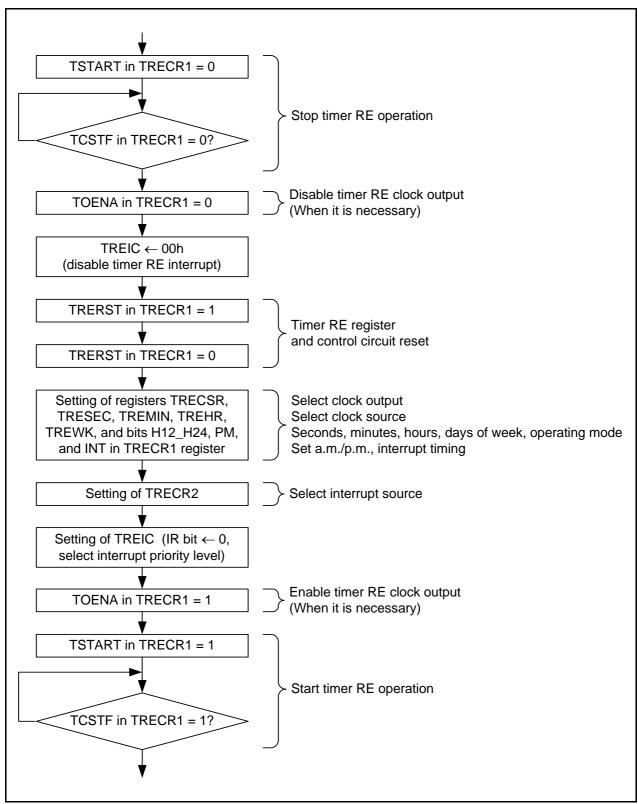
Figure 36.6 Setting Example in Real-Time Clock Mode
