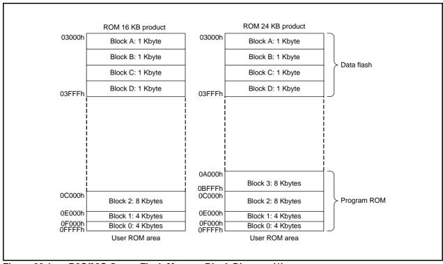
Figure 33.1 R8C/38C Group Flash Memory Block Diagram (1)
