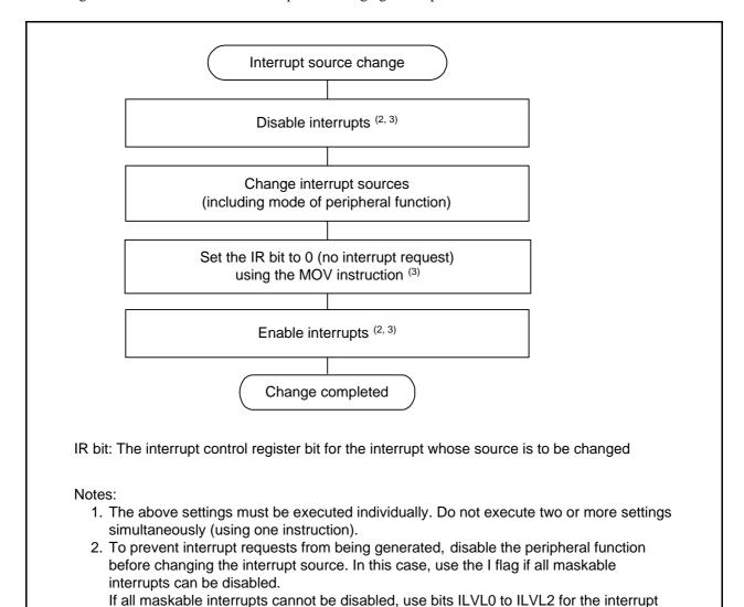
Figure 36.1 Procedure Example for Changing Interrupt Sources
