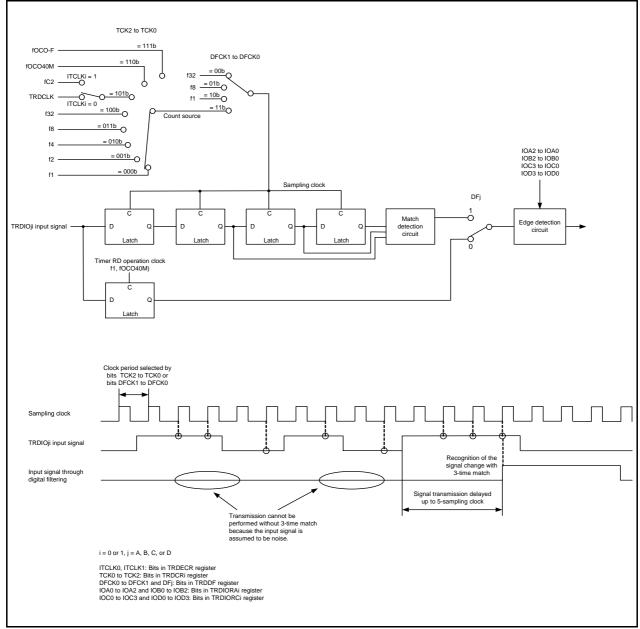
Figure 20.9 Block Diagram of Digital Filter
