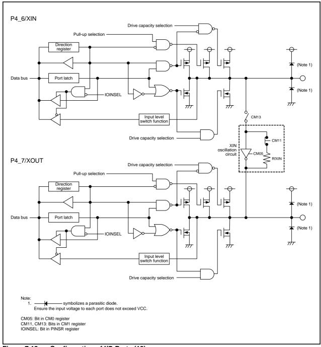
Figure 7.12 Configuration of I/O Ports (12)
