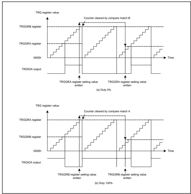
Figure 23.15 Operating Example (2) in PWM Mode
