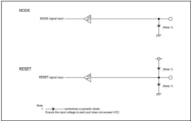
Figure 7.22 Configuration of I/O Pins
