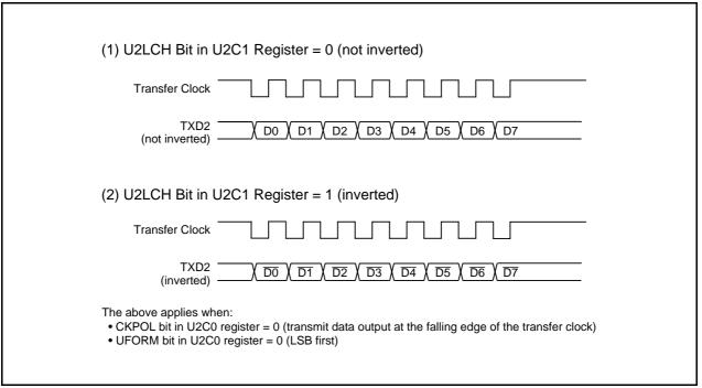
Figure 25.6 Serial Data Logic Switching
