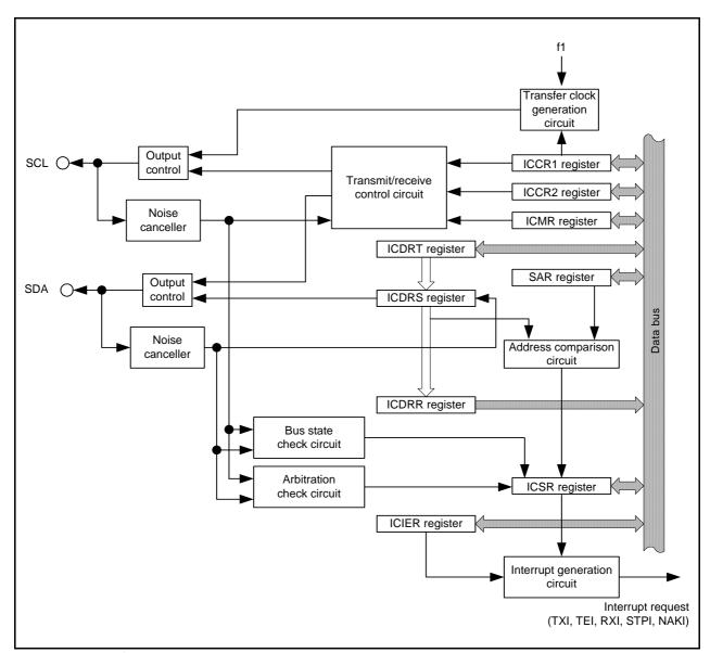
Figure 28.1 I<sup>2</sup>C bus interface Block Diagram
