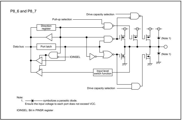
Figure 7.20 Configuration of I/O Ports (20)
