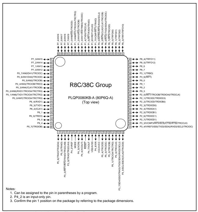
Figure 1.3 Pin Assignment (Top View)
