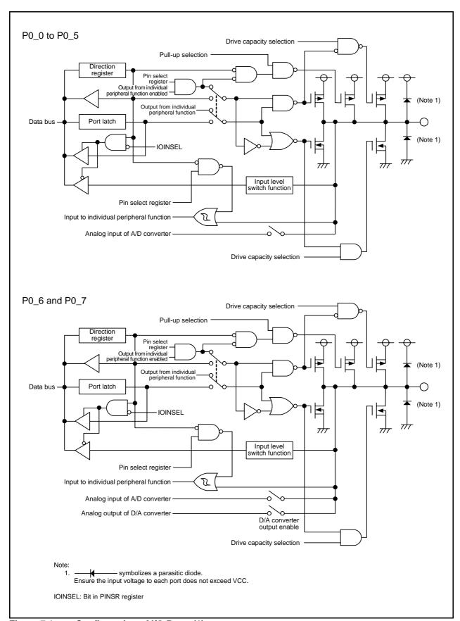
Figure 7.1 Configuration of I/O Ports (1)
