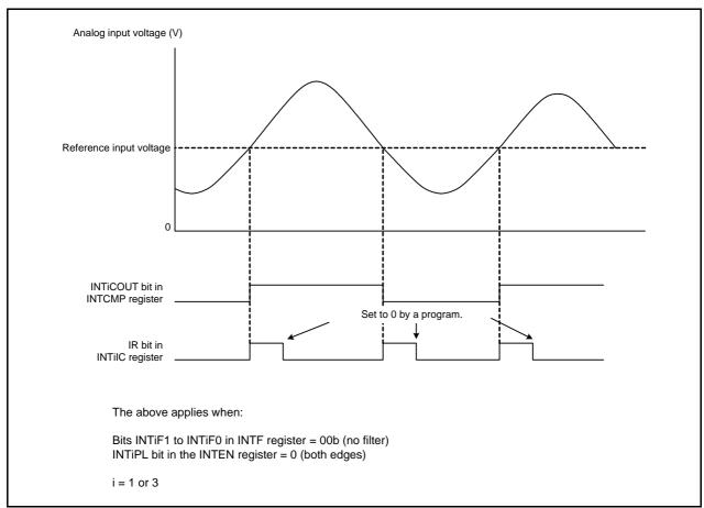
Figure 32.2 Operating Example of Comparator Bi (i = 1 or 3)
