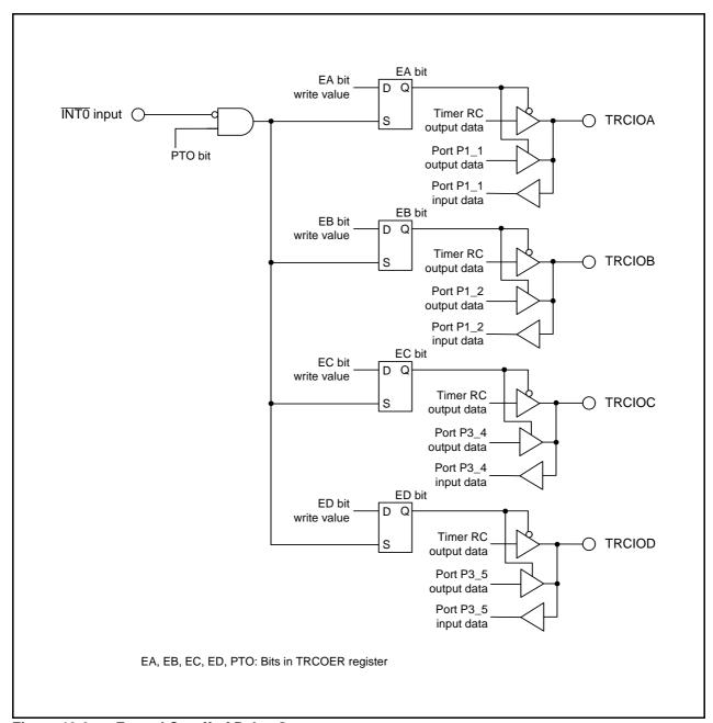
Figure 19.6 Forced Cutoff of Pulse Output
