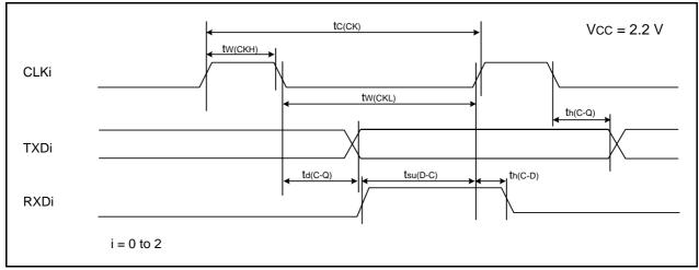
Figure 35.21 Serial Interface Timing Diagram when Vcc = 2.2 V
