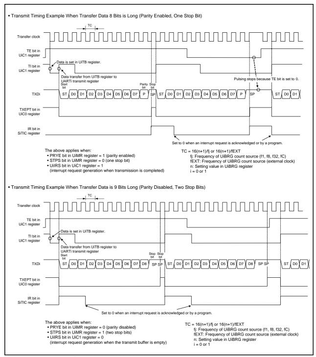
Figure 24.6 Transmit Timing in UART Mode
