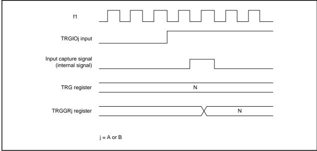
Figure 23.7 Input-Capture Input Signal Timing
