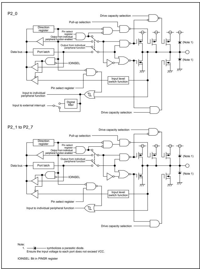
Figure 7.5 Configuration of I/O Ports (5)
