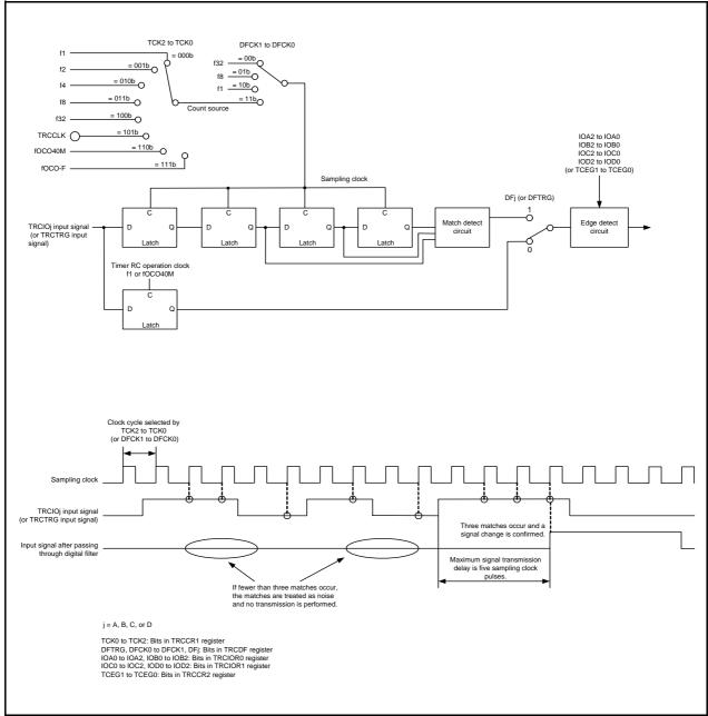
Figure 19.5 Digital Filter Block Diagram
