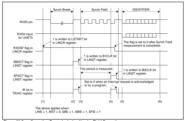
Figure 29.5 Operating Example during Header Field Reception
