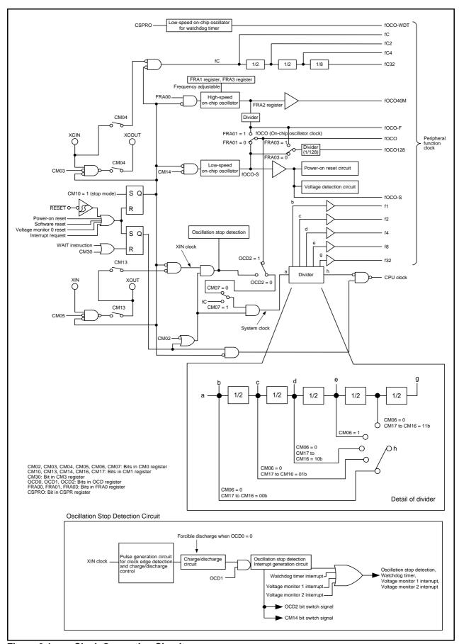
Figure 9.1 Clock Generation Circuit
