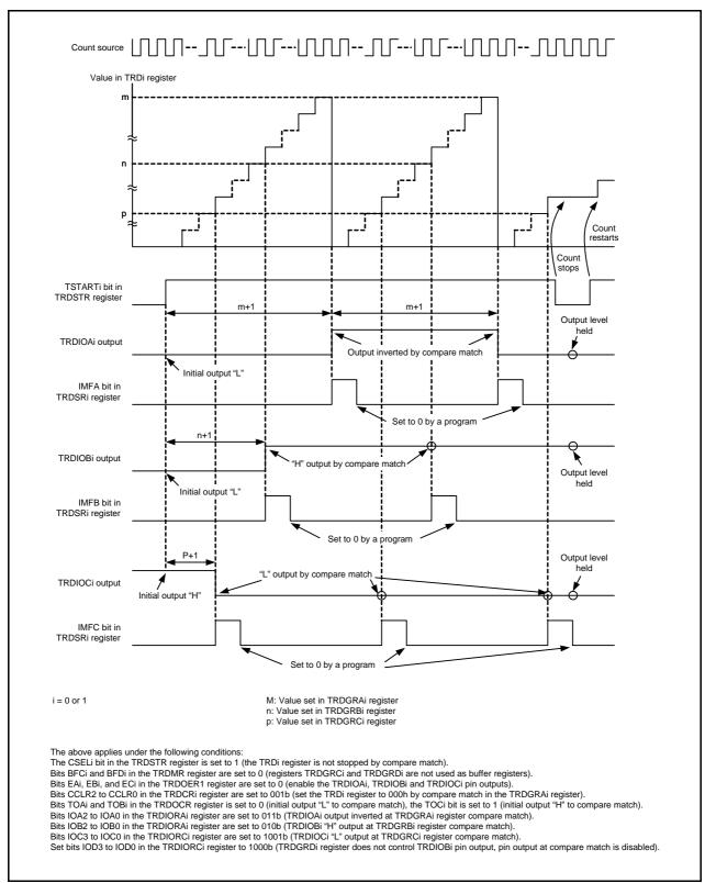
Figure 20.11 Operating Example of Output Compare Function
