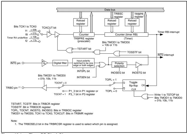
Figure 18.1 Timer RB Block Diagram
