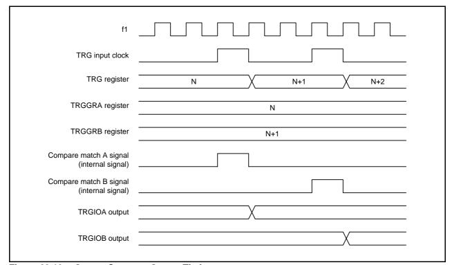
Figure 23.10 Output-Compare Output Timing
