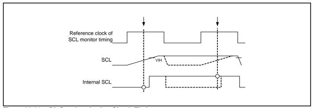
Figure 28.21 Bit Synchronization Circuit Timing
