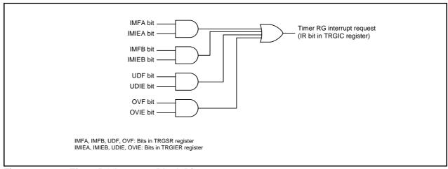
Figure 23.21 Timer RG Interrupt Block Diagram
