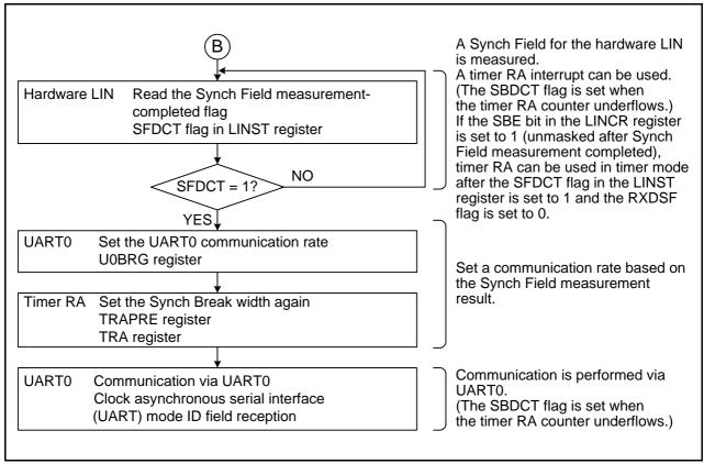
Figure 29.8 Header Field Reception Flowchart Example (3)
