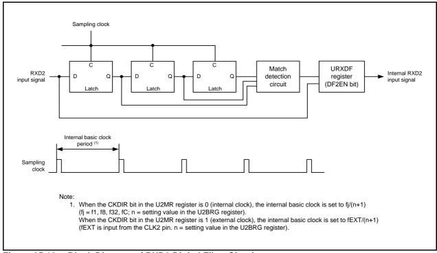
Figure 25.12 Block Diagram of RXD2 Digital Filter Circuit
