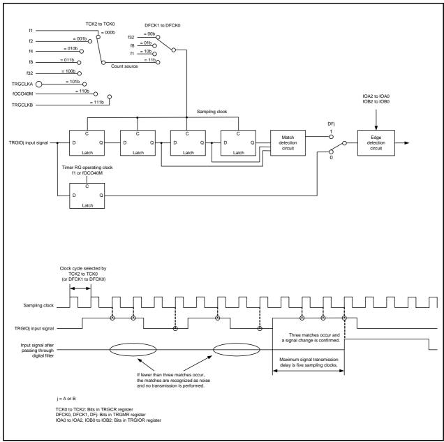
Figure 23.5 Digital Filter Block Diagram
