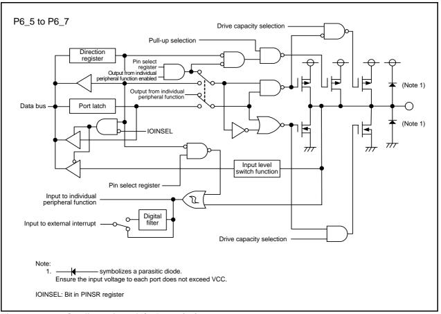
Figure 7.17 Configuration of I/O Ports (17)
