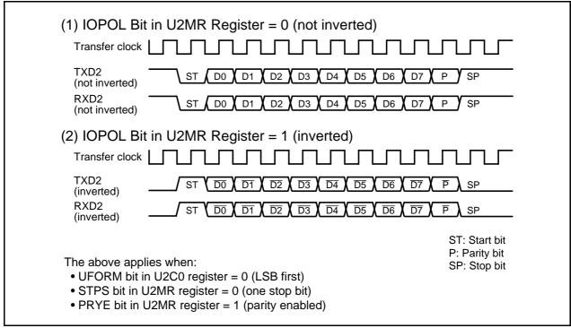
Figure 25.11 TXD and RXD I/O Inversion
