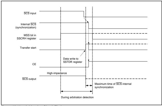
Figure 27.13 Arbitration Check Timing
