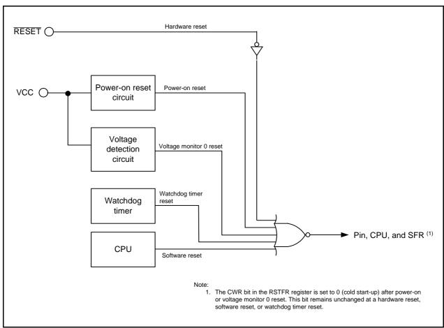
Figure 5.1 Block Diagram of Reset Circuit
