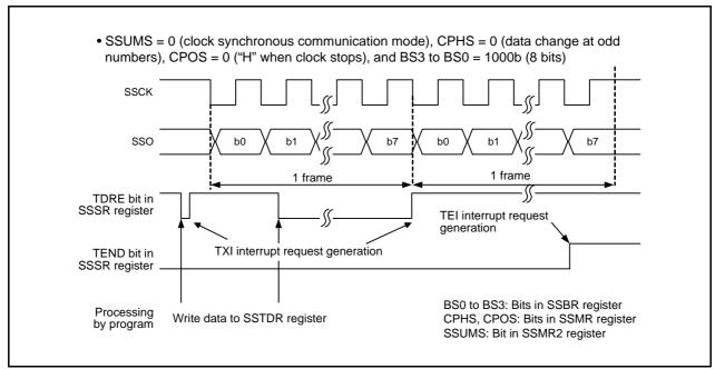
Figure 27.5 Example of Synchronous Serial Communication Unit Operation for Data
