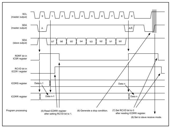
Figure 28.8 Operating Timing in Master Receive Mode (I<sup>2</sup>C bus Interface Mode) (2)
