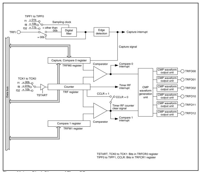
Figure 22.1 Block Diagram of Timer RF
