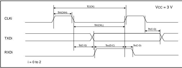
Figure 35.16 Serial Interface Timing Diagram when Vcc = 3 V
