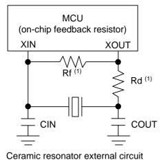
When CM05 bit in CM0 register is set to 1 (XIN clock stops), CM11 bit in CM1 register is set to 1 (internal feedback resistor disabled), and the CM13 bit is set to 1 (XIN-XOUT pin)
