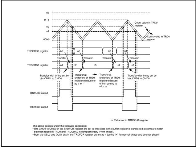
Figure 20.27 Operation when Value in Buffer Register ≥ Value in TRDGRA0 Register in Complementary PWM Mode
