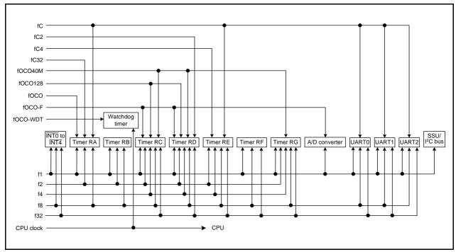
Figure 9.2 Peripheral Function Clock
