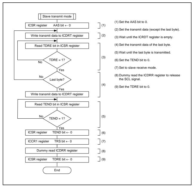
Figure 28.18 Register Setting Example in Slave Transmit Mode (I<sup>2</sup>C bus Interface Mode)
