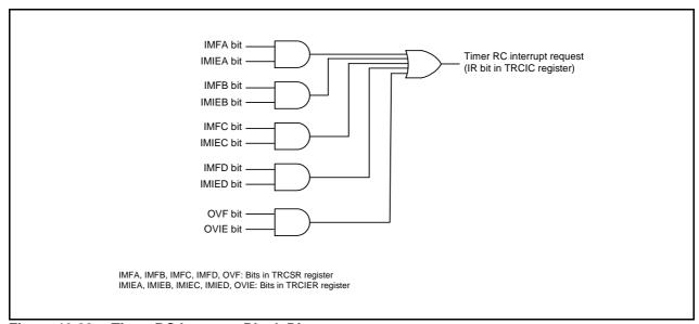
Figure 19.20 Timer RC Interrupt Block Diagram
