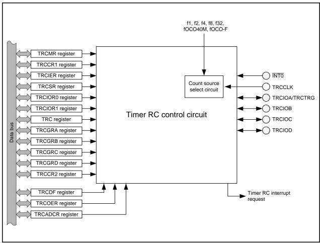
Figure 19.1 Timer RC Block Diagram
