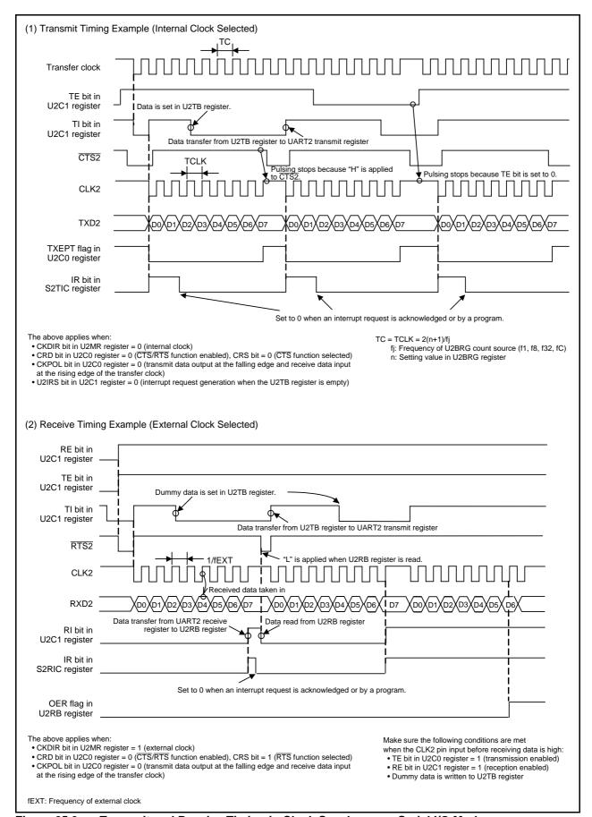
Figure 25.3 Transmit and Receive Timing in Clock Synchronous Serial I/O Mode
