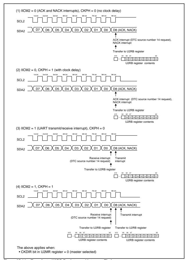
Figure 25.14 Transfer to U2RB Register and Interrupt Timing
