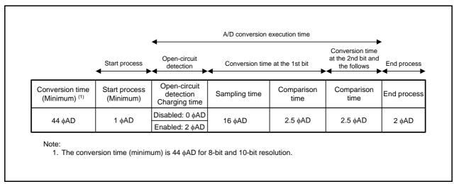
Figure 30.3 A/D Conversion Cycles ( $\phi AD = fAD$ )
