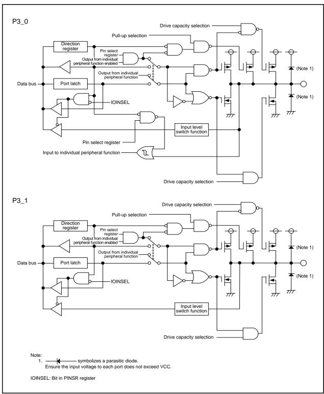
Figure 7.6 Configuration of I/O Ports (6)
