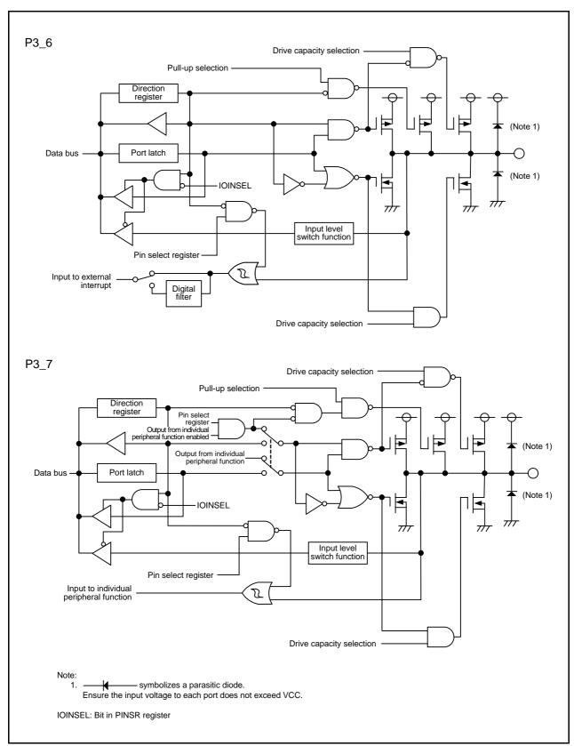
Figure 7.9 Configuration of I/O Ports (9)
