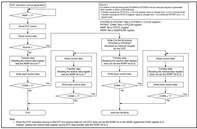
Figure 15.5 DTC Internal Operation Flowchart When DTC Activation Source is SSU/I<sup>2</sup>C bus Receive Data Full
