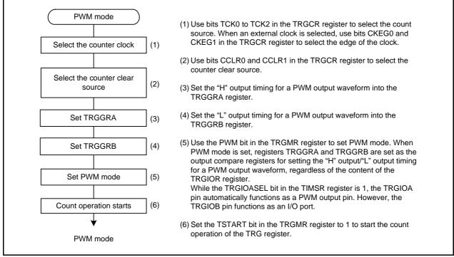
Figure 23.13 Procedure Example for Setting PWM Mode
