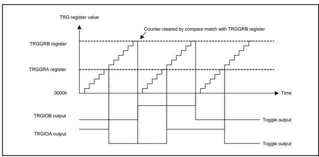
Figure 23.12 Operating Example of Toggle Output
