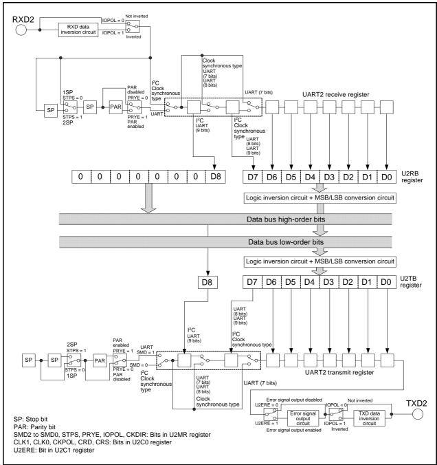
Figure 25.2 Block Diagram of UART2 Transmit/Receive Unit
