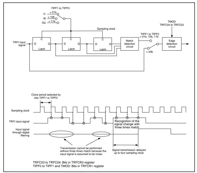
Figure 22.5 Block Diagram of Digital Filter
