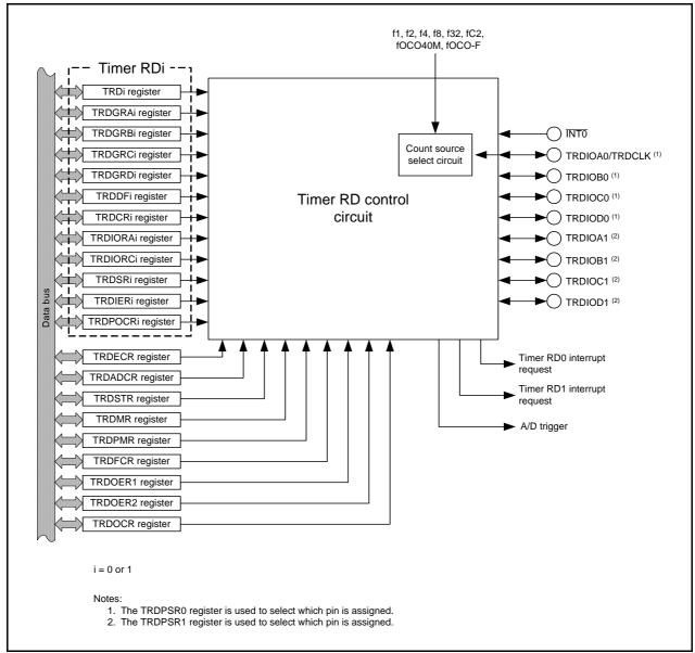
Figure 20.1 Timer RD Block Diagram
