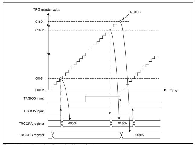
Figure 23.8 Operating Example of Input Capture
