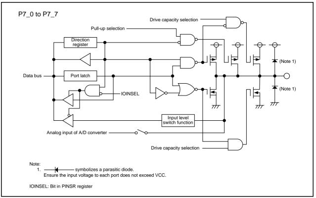
Figure 7.18 Configuration of I/O Ports (18)
