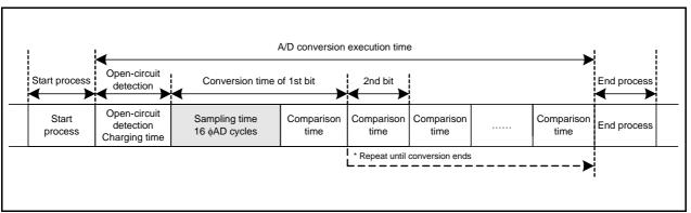
Figure 30.2 Timing Diagram of A/D Conversion
