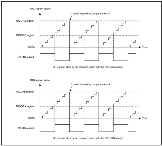
Figure 23.14 Operating Example (1) in PWM Mode
