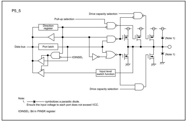
Figure 7.14 Configuration of I/O Ports (14)
