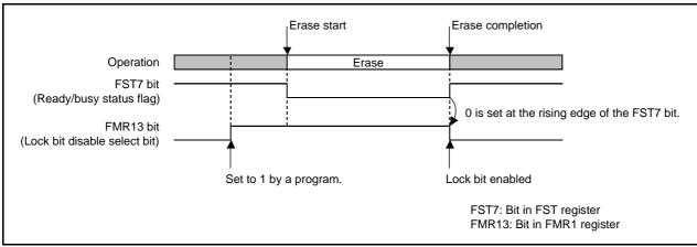
Figure 33.8 FMR13 Bit Operation Timing
