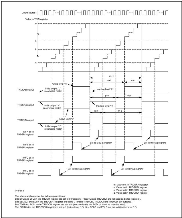
Figure 20.15 Operating Example of PWM Mode
