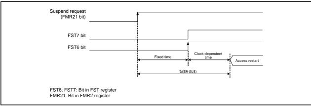
Figure 35.2 Time delay until Suspend
