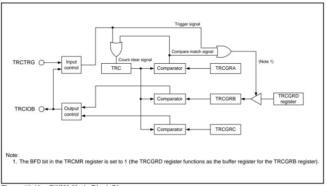
Figure 19.16 PWM2 Mode Block Diagram
