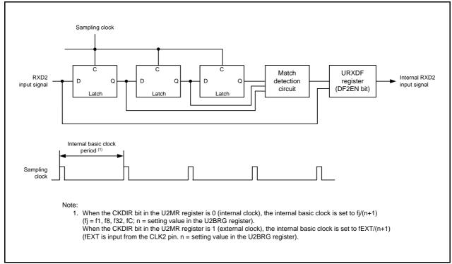
Figure 25.22 Block Diagram of RXD2 Digital Filter Circuit
