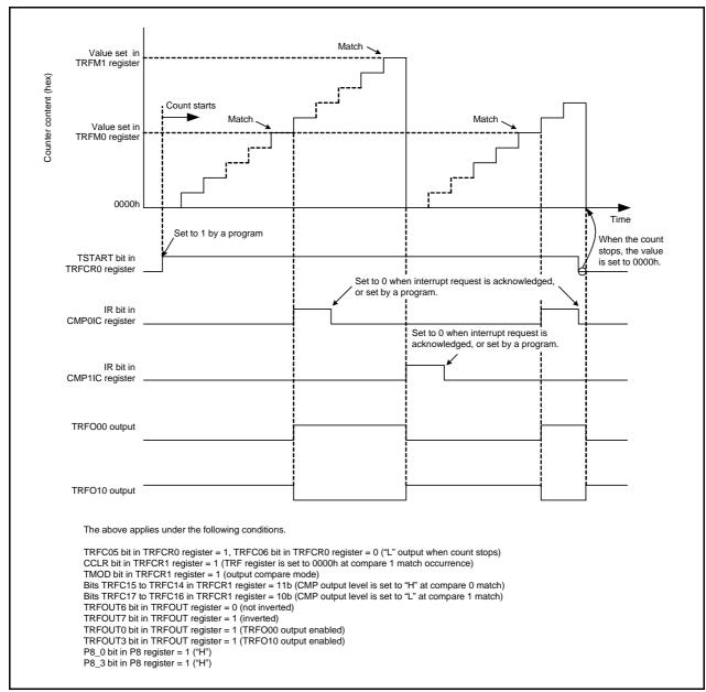
Figure 22.6 Operating Example in Output Compare Mode
