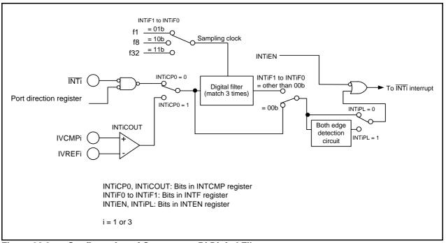
Figure 32.3 Configuration of Comparator Bi Digital Filter
