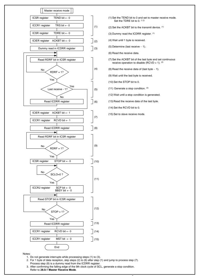
Figure 28.17 Register Setting Example in Master Receive Mode (I<sup>2</sup>C bus Interface Mode)
