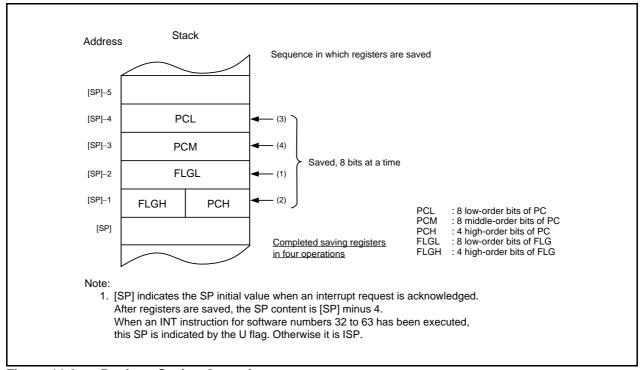
Figure 11.6 Register Saving Operation
