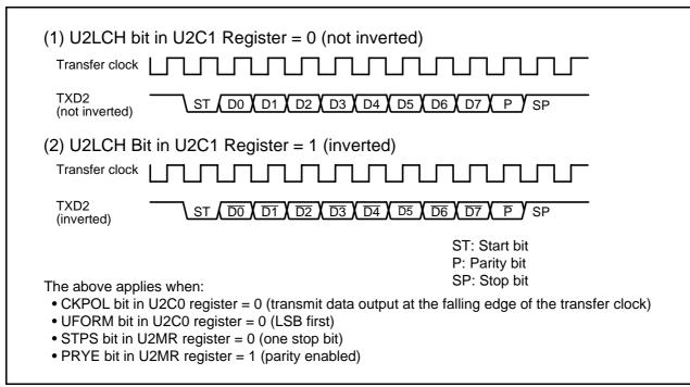
Figure 25.10 Serial Data Logic Switching
