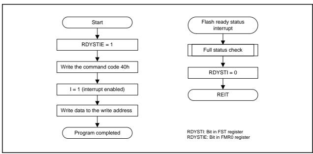
Figure 33.10 Program Flowchart (Flash Ready Status Interrupt Enabled)
