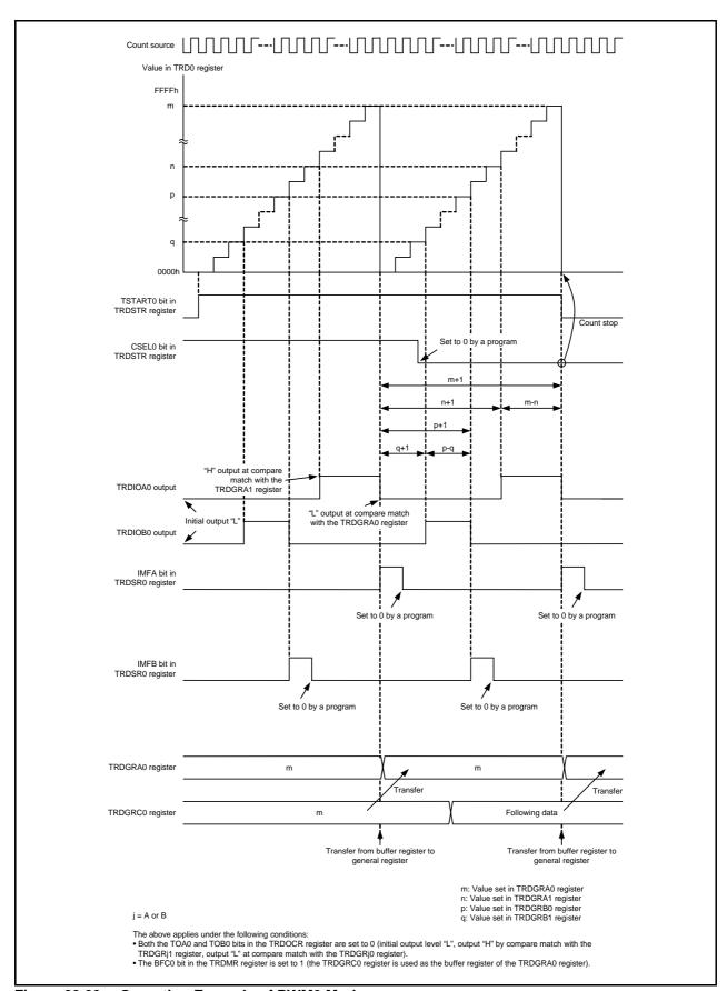
Figure 20.23 Operating Example of PWM3 Mode
