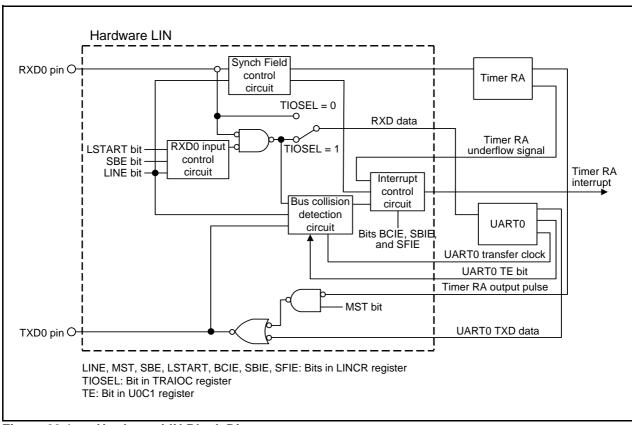
Figure 29.1 Hardware LIN Block Diagram
