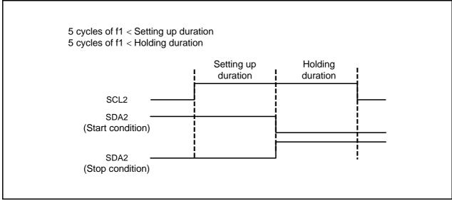
Figure 25.15 Detection of Start and Stop Conditions
