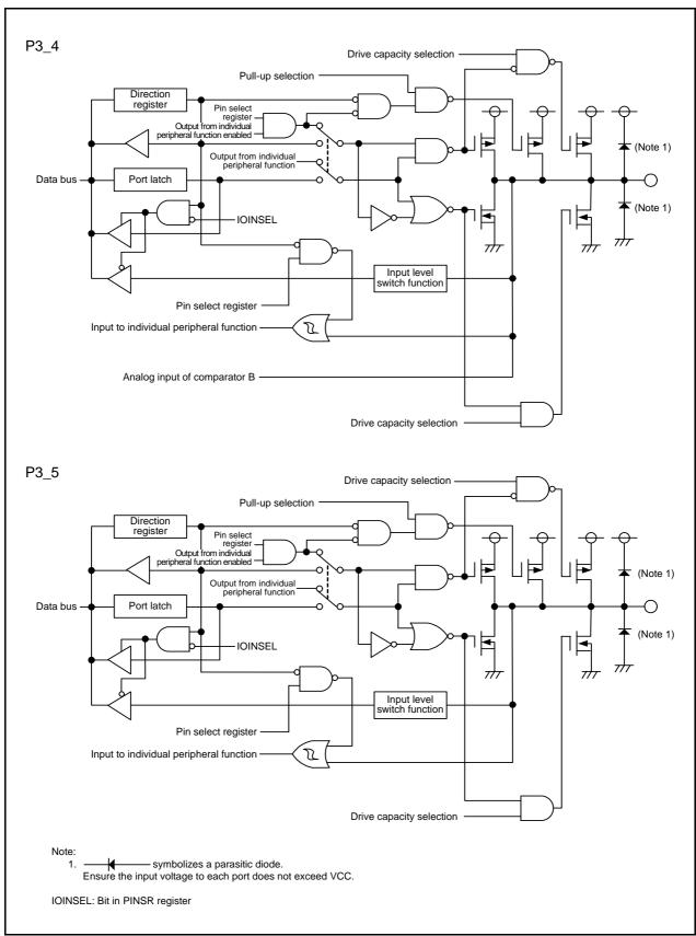
Figure 7.8 Configuration of I/O Ports (8)
