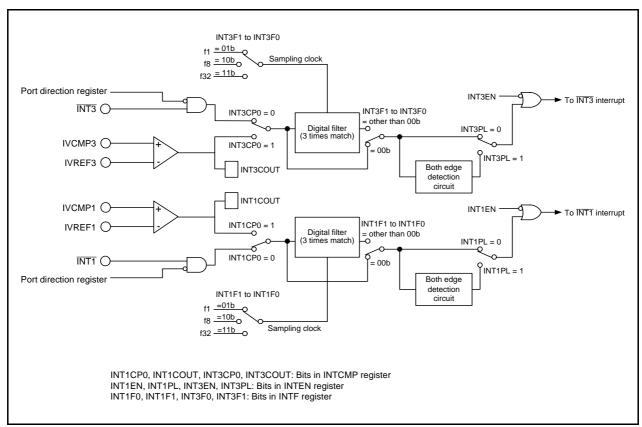
Figure 32.1 Comparator B Block Diagram
