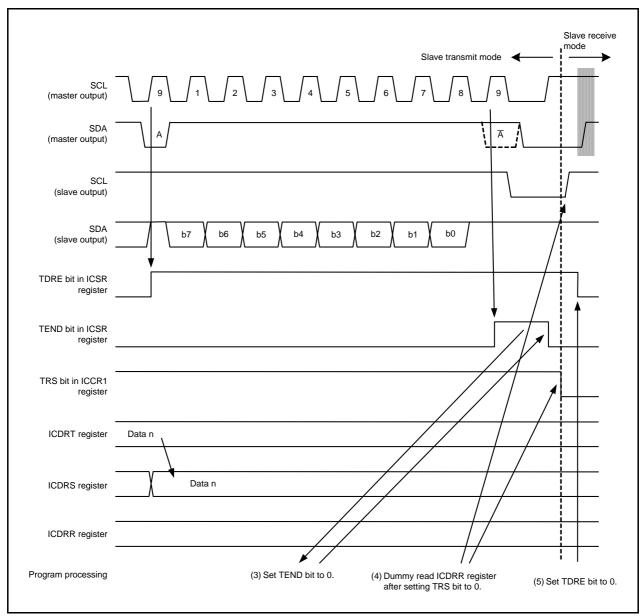
Figure 28.10 Operating Timing in Slave Transmit Mode (I<sup>2</sup>C bus Interface Mode) (2)
