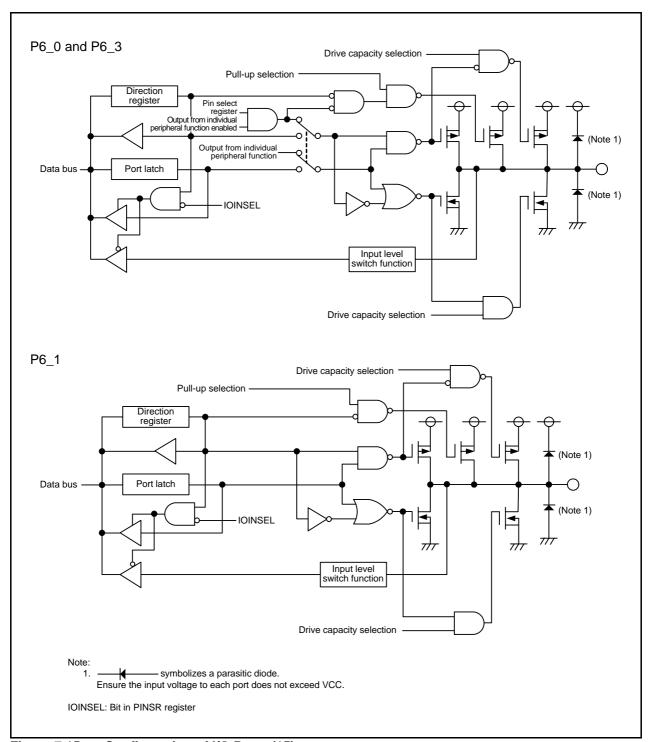
Figure 7.15 Configuration of I/O Ports (15)
