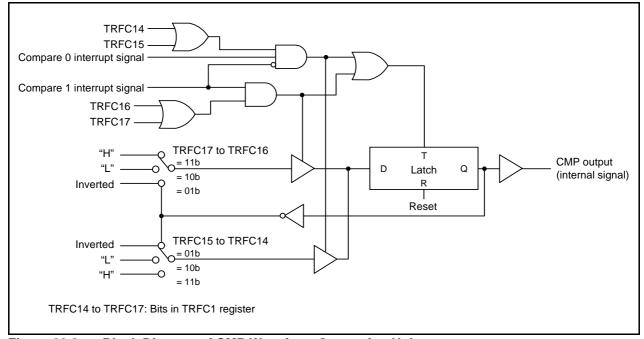
Figure 22.2 Block Diagram of CMP Waveform Generation Unit
