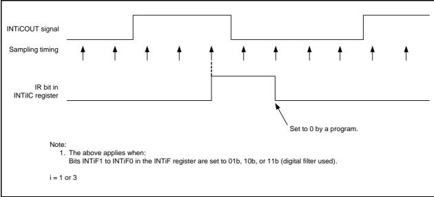
Figure 32.4 Operating Example of Comparator Bi Digital Filter
