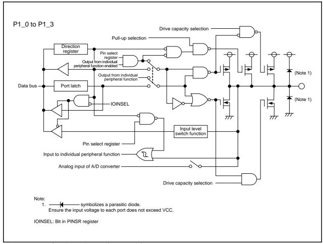
Figure 7.2 Configuration of I/O Ports (2)
