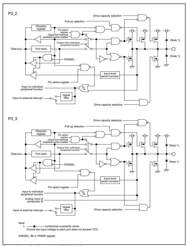
Figure 7.7 Configuration of I/O Ports (7)
