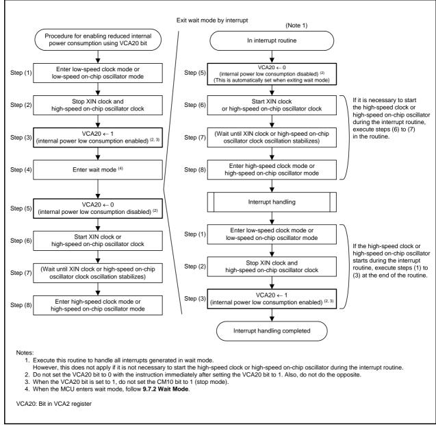
Figure 34.1 Handling Procedure for Reducing Internal Power Consumption Using VCA20 Bit
