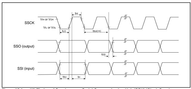
Figure 35.6 I/O Timing of Synchronous Serial Communication Unit (SSU) (Clock Synchronous Communication Mode)
