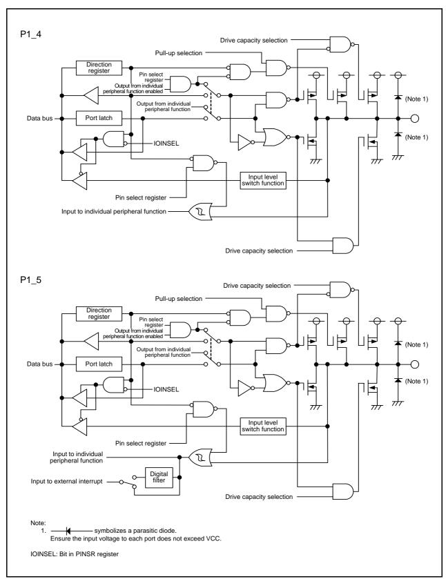
Figure 7.3 Configuration of I/O Ports (3)
