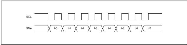
Figure 28.13 Transfer Format of Clock Synchronous Serial Format
