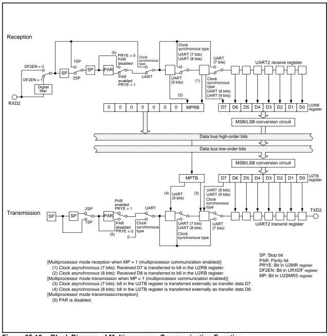
Figure 25.18 Block Diagram of Multiprocessor Communication Function
