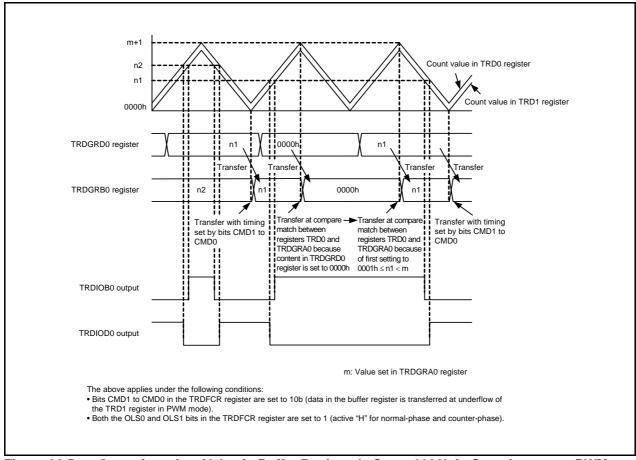
Figure 36.5 Operation when Value in Buffer Register Is Set to 0000h in Complementary PWM Mode
