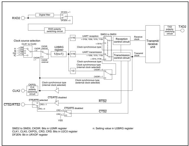
Figure 25.1 UART2 Block Diagram
