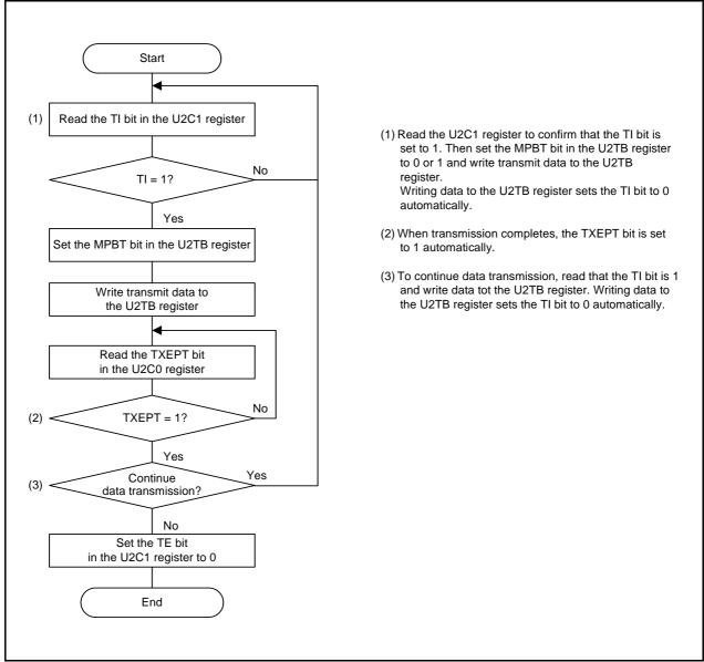
Figure 25.19 Sample Flowchart of Multiprocessor Data Transmission
