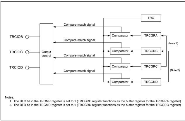
Figure 19.13 PWM Mode Block Diagram
