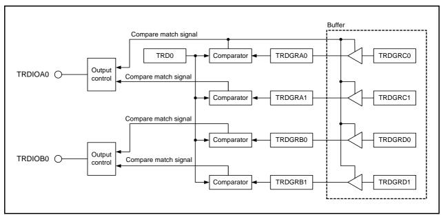
Figure 20.22 Block Diagram of PWM3 Mode
