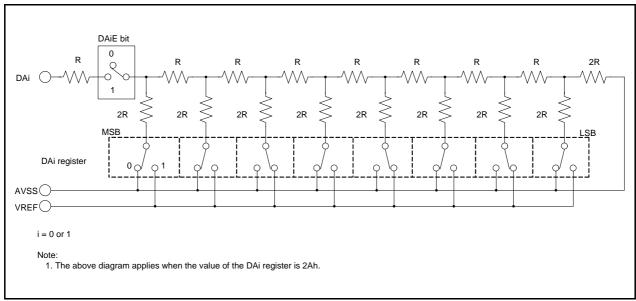
Figure 31.2 D/A Converter Equivalent Circuit
