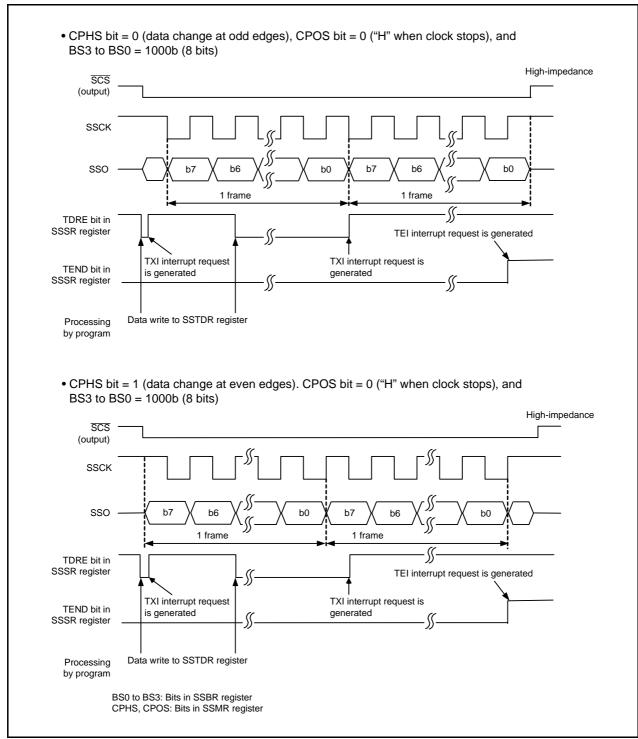
Figure 27.11 Example of Synchronous Serial Communication Unit Operation during Data
