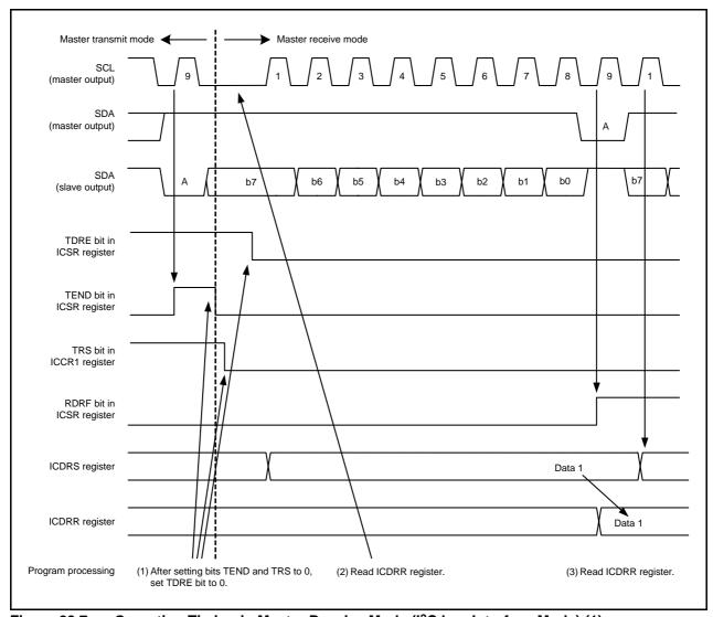
Figure 28.7 Operating Timing in Master Receive Mode (I<sup>2</sup>C bus Interface Mode) (1)
