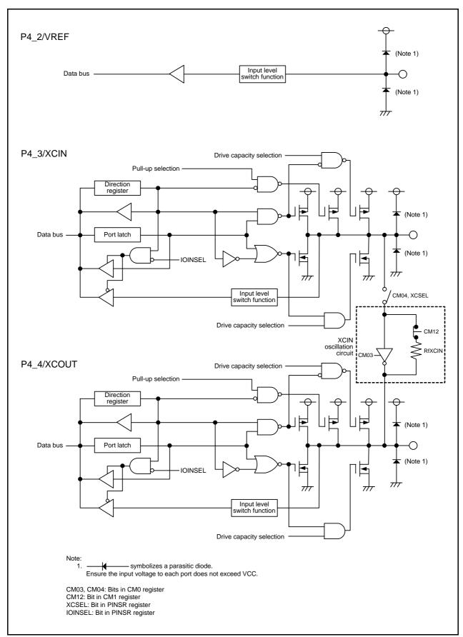
Figure 7.10 Configuration of I/O Ports (10)
