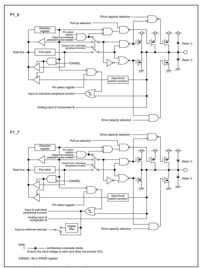
Figure 7.4 Configuration of I/O Ports (4)
