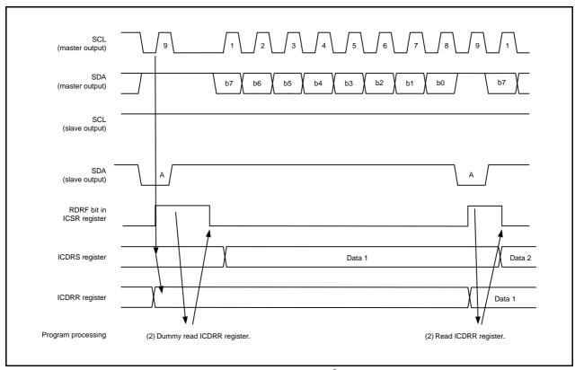
Figure 28.11 Operating Timing in Slave Receive Mode (I<sup>2</sup>C bus Interface Mode) (1)
