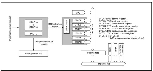
Figure 15.1 DTC Block Diagram
