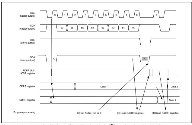
Figure 28.12 Operating Timing in Slave Receive Mode (I<sup>2</sup>C bus Interface Mode) (2)
