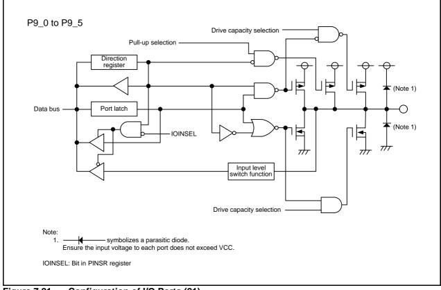
Figure 7.21 Configuration of I/O Ports (21)
