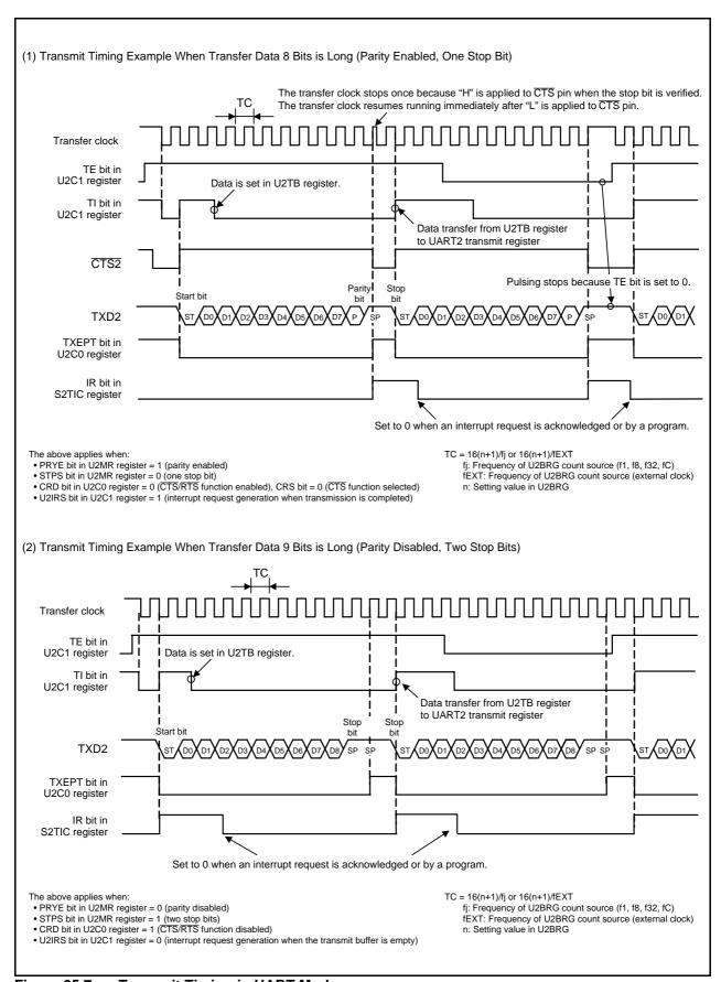
Figure 25.7 Transmit Timing in UART Mode
