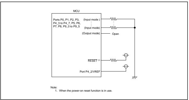
Figure 7.23 Unassigned Pin Handling
