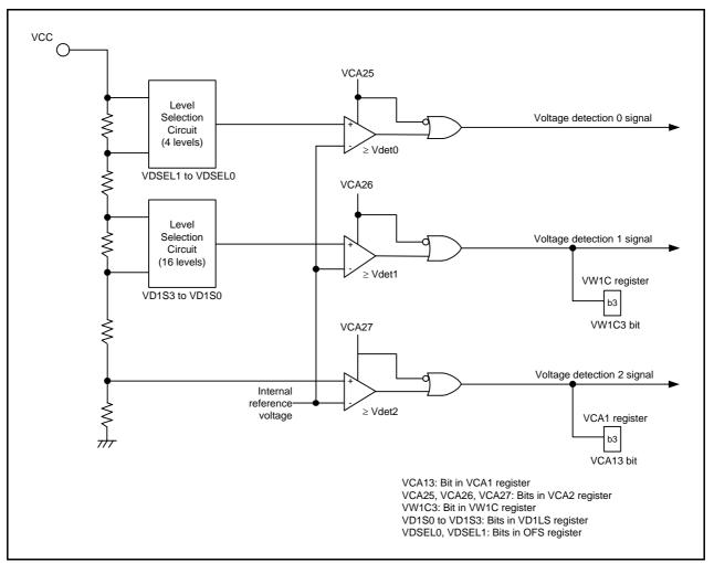
Figure 6.1 Voltage Detection Circuit Block Diagram
