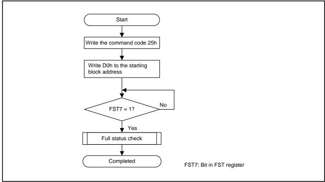
Figure 33.16 Block Blank Check Flowchart
