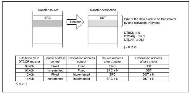
Figure 15.8 Data Transfers in Normal Mode
