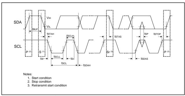
Figure 35.7 I/O Timing of I<sup>2</sup>C bus Interface
