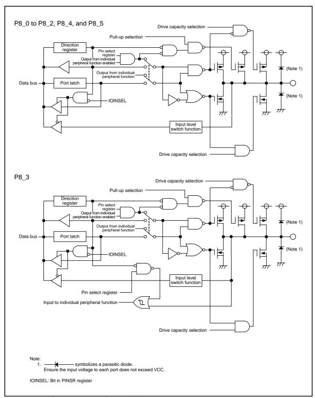
Figure 7.19 Configuration of I/O Ports (19)
