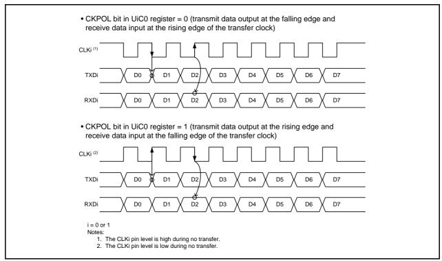
Figure 24.4 Transfer Clock Polarity
