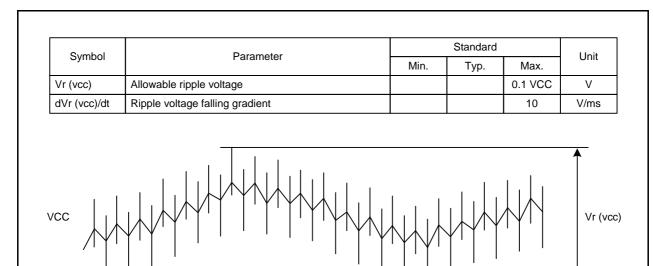
Figure 36.8 Definition of ripple voltage
