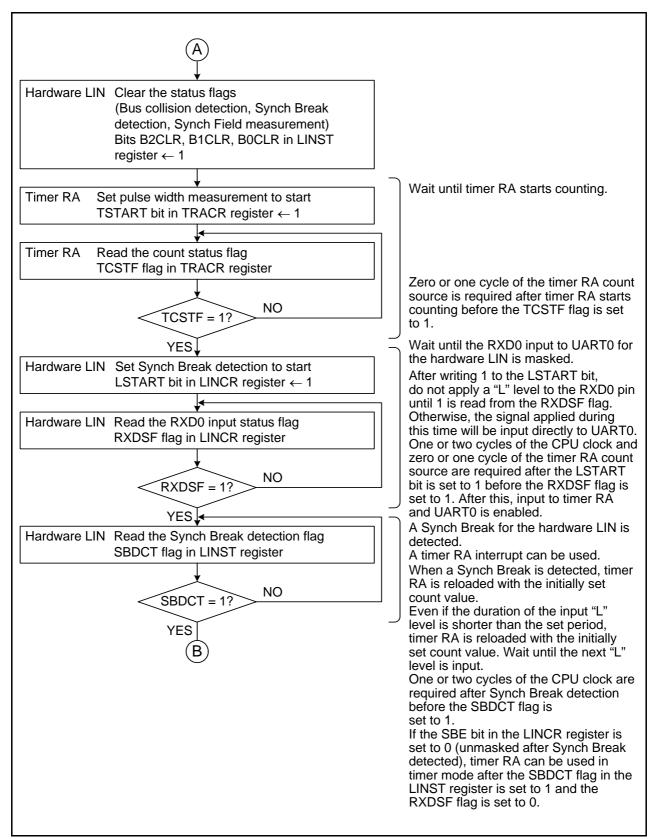
Figure 29.7 Header Field Reception Flowchart Example (2)
