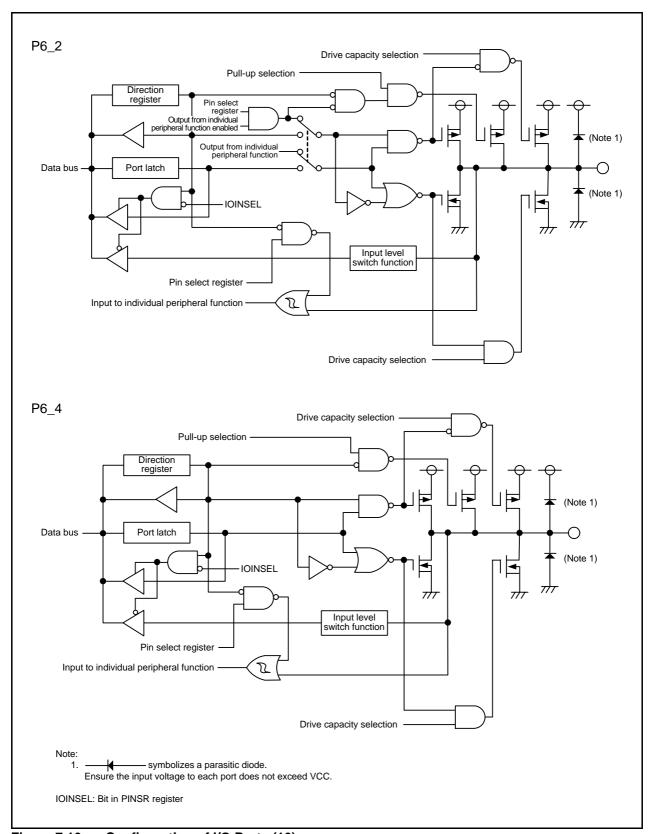
Figure 7.16 Configuration of I/O Ports (16)
