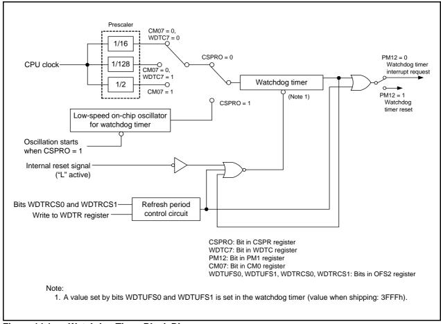
Figure 14.1 Watchdog Timer Block Diagram
