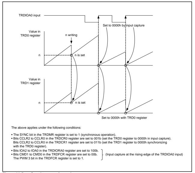
Figure 20.5 Synchronous Operation
