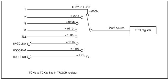
Figure 23.2 Count Source Block Diagram
