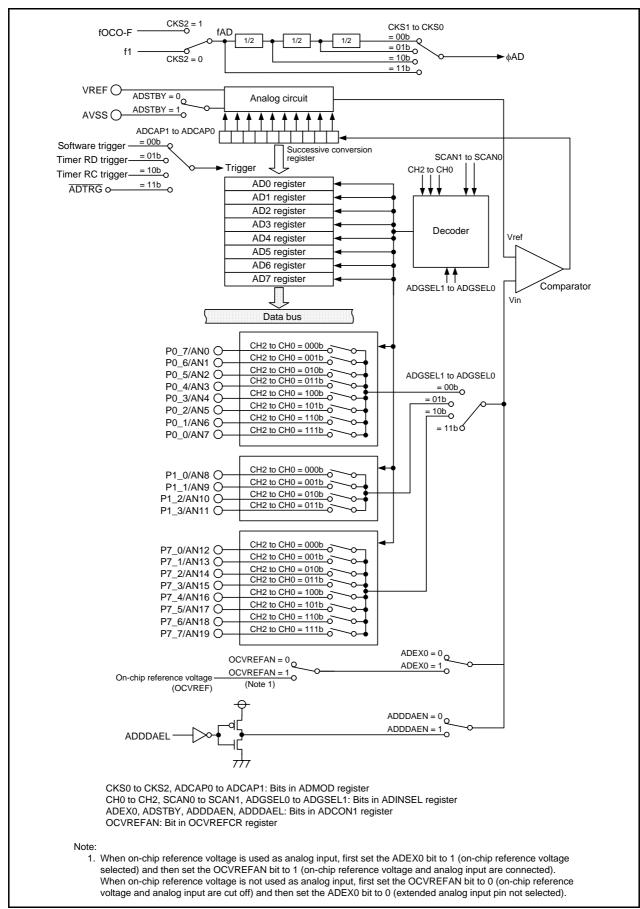
Figure 30.1 Block Diagram of A/D Converter
