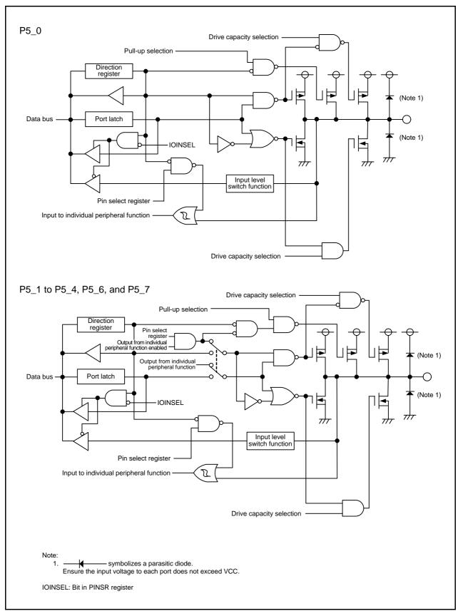
Figure 7.13 Configuration of I/O Ports (13)
