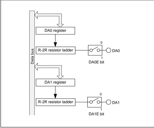
Figure 31.1 D/A Converter Block Diagram
