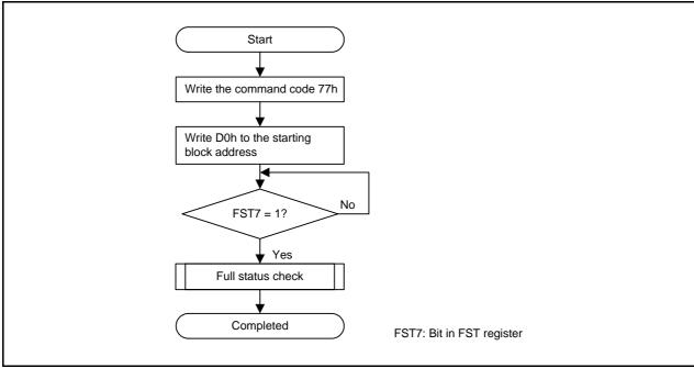
Figure 33.14 Lock Bit Program Flowchart
