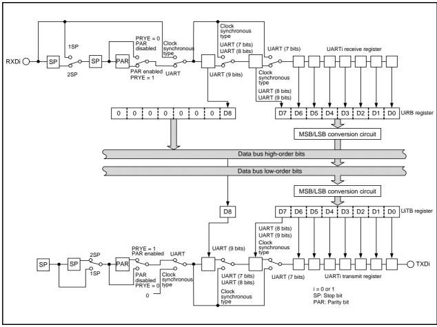
Figure 24.2 Block Diagram of UARTi Transmit/Receive Unit
