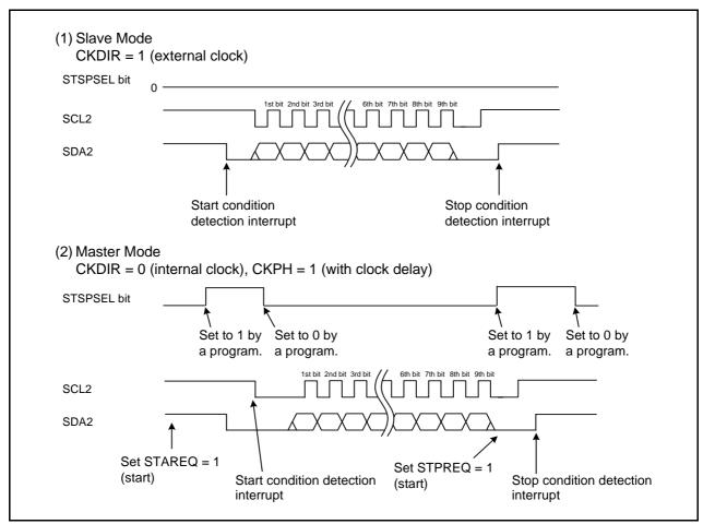
Figure 25.16 STSPSEL Bit Functions
