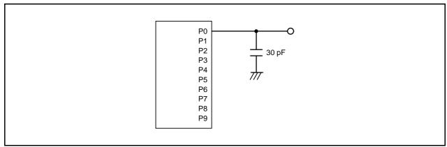
Figure 35.1 Ports P0 to P9 Timing Measurement Circuit
