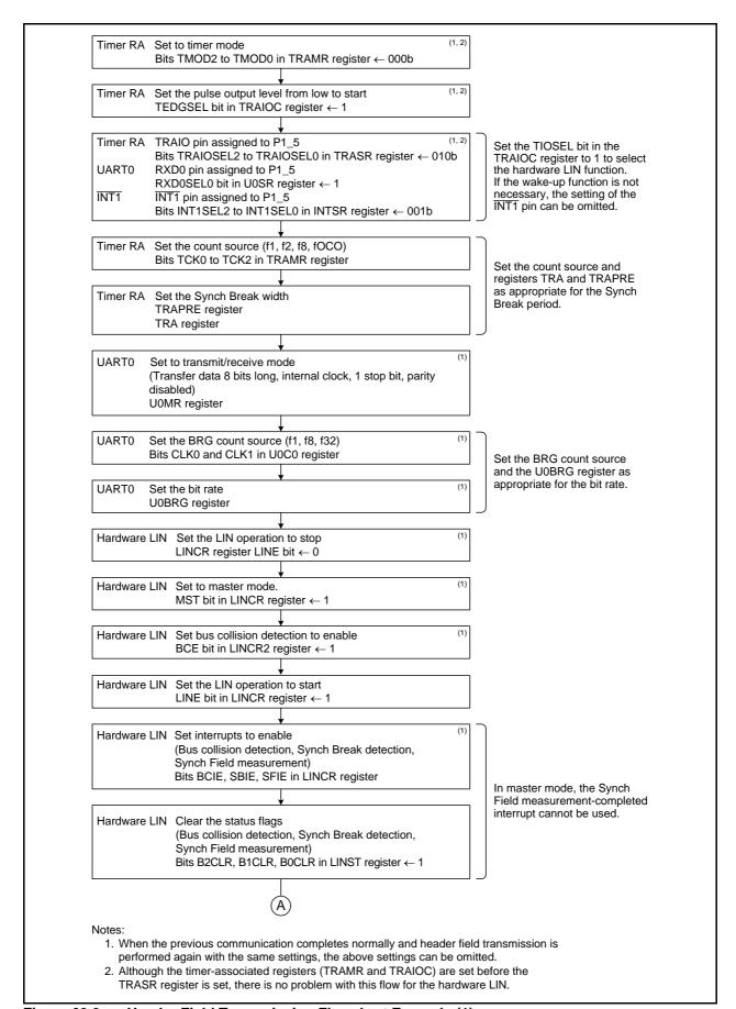
Figure 29.3 Header Field Transmission Flowchart Example (1)
