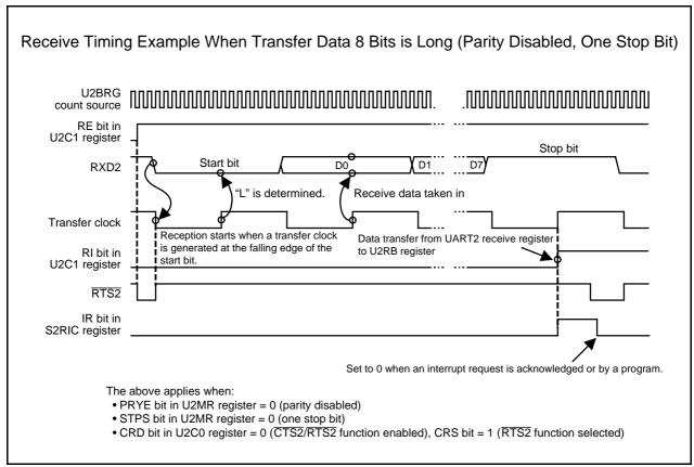
Figure 25.8 Receive Timing in UART Mode
