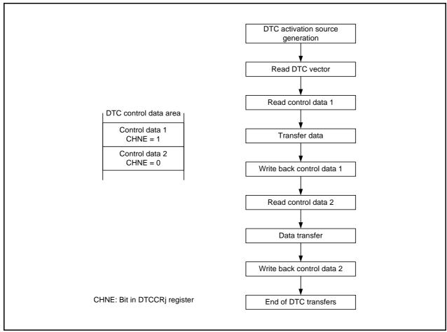
Figure 15.10 Flow of Chain Transfers
