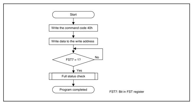
Figure 33.9 Program Flowchart (Flash Ready Status Interrupt Disabled)
