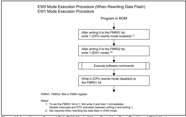
Figure 33.6 How to Set and Exit EW0 Mode (When Rewriting Data Flash) and EW1 Mode
